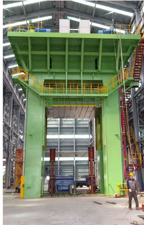
10,000 Ton Hydraulic Press
